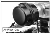
Figure 2. Air filter attached to cylinder head.
